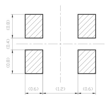
Note) Please reserve a large ground pattern on the PCB where the oscillator is installed.
