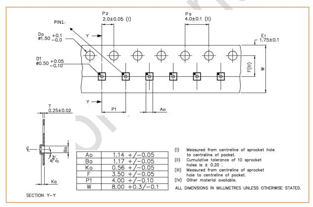
Figure 5 Tape and Reel Dimensions
