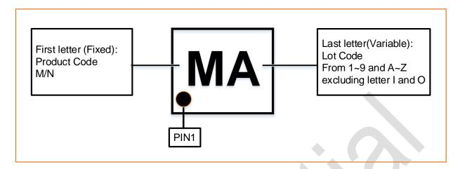
Figure 4 Marking Specification(Top View)
