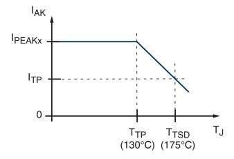
Figure 14. Peak Regulating Current vs. TJ
