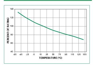
Re-rating depicted in this curve is in addition to the standard re-rating of 20% for continuous
