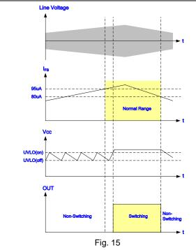
Over Voltage Protection on FB pin (FB OVP) – Auto Recovery
