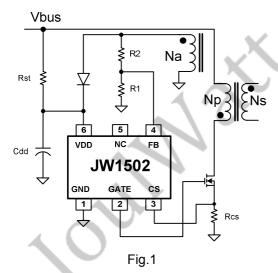
Once JW1502 enters very low frequency FM (Frequency Modulation) mode, the operating current is reduced to be 0.5mA typically, which helps to reduce the standby power loss.
