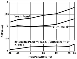
FIGURE 11. DRIVER SKEW vs TEMPERATURE
