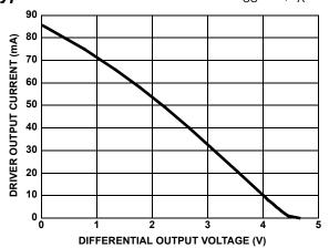
FIGURE 6. DRIVER OUTPUT CURRENT VS DIFFERENTIAL OUTPUT VOLTAGE
