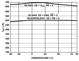
FIGURE 9. SUPPLY CURRENT vs TEMPERATURE
