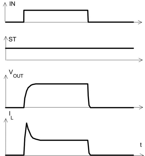
The initial peak current should be limited by the lamp and not by the current limit of the device.
