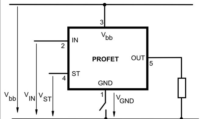
Any kind of load. In case of Input=high is  $V_{OUT} \approx V_{IN} - V_{IN(T+)}$ . Due to  $V_{GND} > 0$ , no  $V_{ST} = \text{low}$  signal available.
