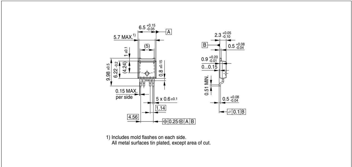
**Figure 1** PG-TO-252 (Plastic Dual Small Outline Package) (RoHS-compliant)
