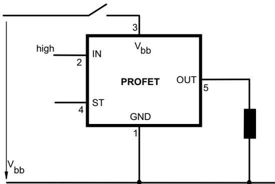
For inductive load currents up to the limits defined by  $Z_L$  (max. ratings and diagram on page 9) each switch is protected against loss of  $V_{bb}$ .
