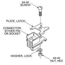
Kit consists of 1 plate, 1 screw, 1 lock washer, 1 hex nut Order 2 kits per connector
