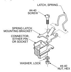
Kit consists of 1 spring, 1 screw, 1 bracket, 1 lock washer, 1 hex nut Order 2 kits per connector Front panel mounting
