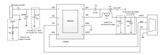
Fig. 5 IP6503S Application Schematic
