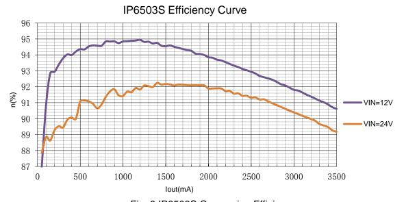
Fig. 3 IP6503S Conversion Efficiency
