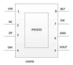
Fig. 2 IP6503S PIN Configuration
