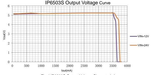
Fig.4 IP6503S Output Voltage Characteristics
