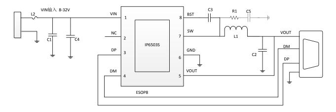
Fig. 1 IP6503S Simplified Schematic
