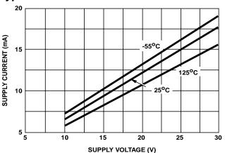
FIGURE 11. SUPPLY CURRENT vs SUPPLY VOLTAGE
