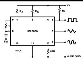
FIGURE 5A. CONNECTIONS FOR FREQUENCY MODULATION
