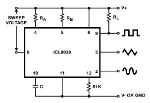
FIGURE 5B. CONNECTIONS FOR FREQUENCY SWEEP FIGURE 5.
