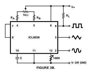
FIGURE 3. POSSIBLE CONNECTIONS FOR THE EXTERNAL TIMING RESISTORS
