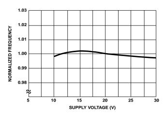
FIGURE 12. FREQUENCY vs SUPPLY VOLTAGE
