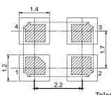
Tolerance: ±0.1 Unit: mm
