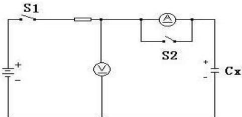
Rs: Protective resistor(1000±100Ω )
