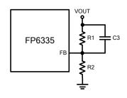
For optimizing the feedforward capacitor, knowing the cross frequency is the first thing. The cross frequency (or the converter bandwidth) can be determined by using a network analyzer. When getting the cross frequency with no feedforward capacitor identified, the value of feedforward capacitor C6 can be calculated with the following equation:
