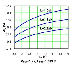
A good compromise value between size and efficiency is to set the peak-to-peak inductor ripple current  $\Delta I_{L}$  equal to 30% of the maximum load current. But setting the peak-to-peak inductor ripple current  $\Delta I_{L}$  between 20%~50% of the maximum load current is also acceptable. Then the inductance can be calculated with the following equation:
