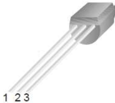
1. Emitter 2. Base 3. Collector TO-92
