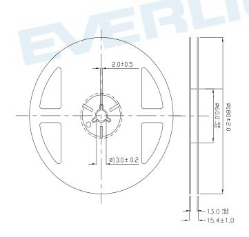
Note: The tolerances unless mentioned are ±0.1, unit=mm
