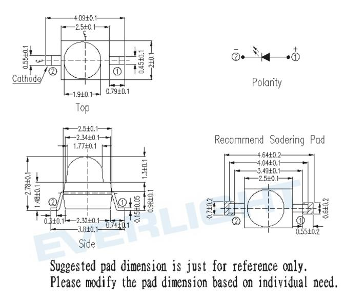
Note: The tolerances unless mentioned are ±0.1, unit=mm.
