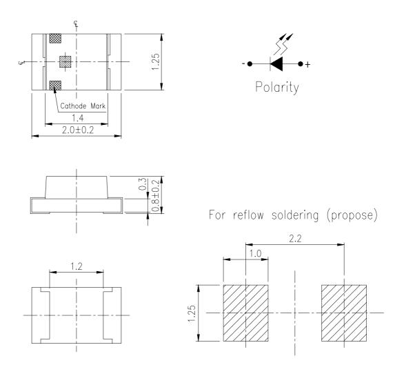
**Note:** The tolerances unless mentioned are  $\pm 0.1$  mm ,Unit = mm
