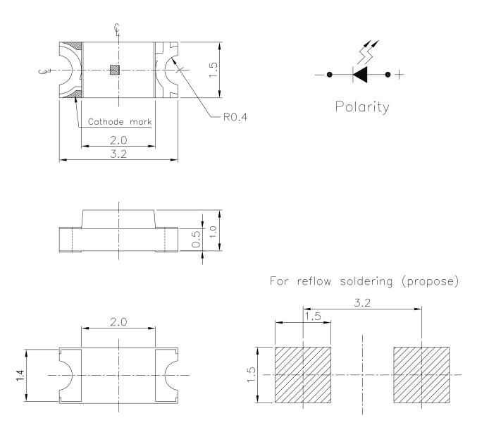
**Note:** Tolerances Unless Dimension is  $\pm 0.1$ mm, Unit = mm
