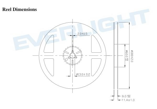
**Note:** The tolerances unless mentioned are  $\pm 0.1$ , Unit = mm.
