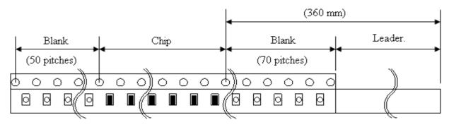
Material of carrier tape : Polystyrene Material of cover tape : Polyester
