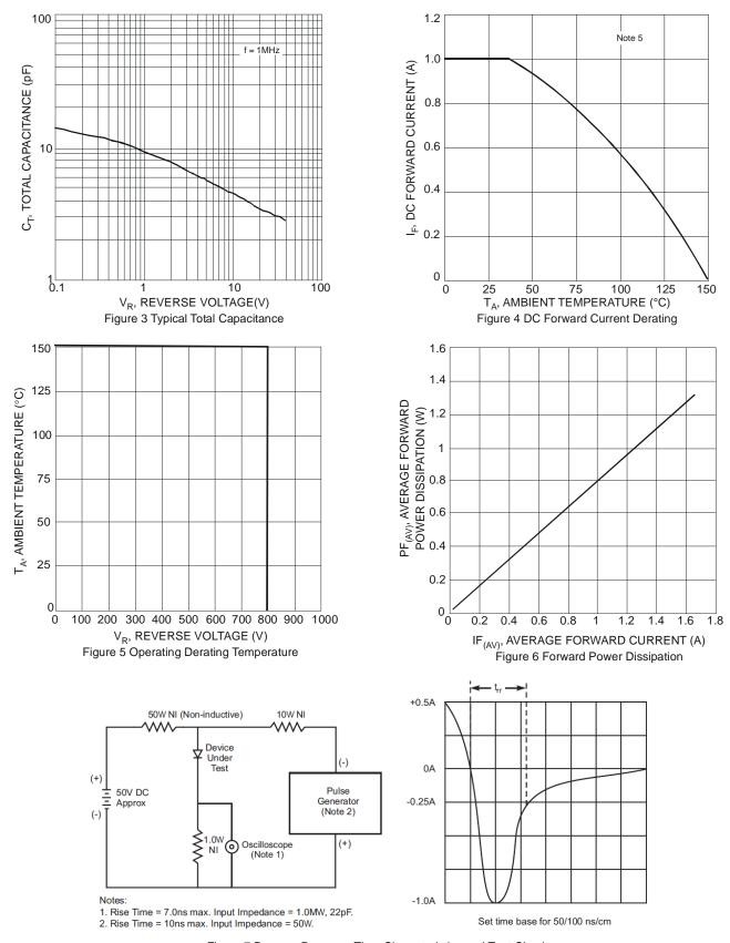
Figure 7 Reverse Recovery Time Characteristics and Test Circuit
