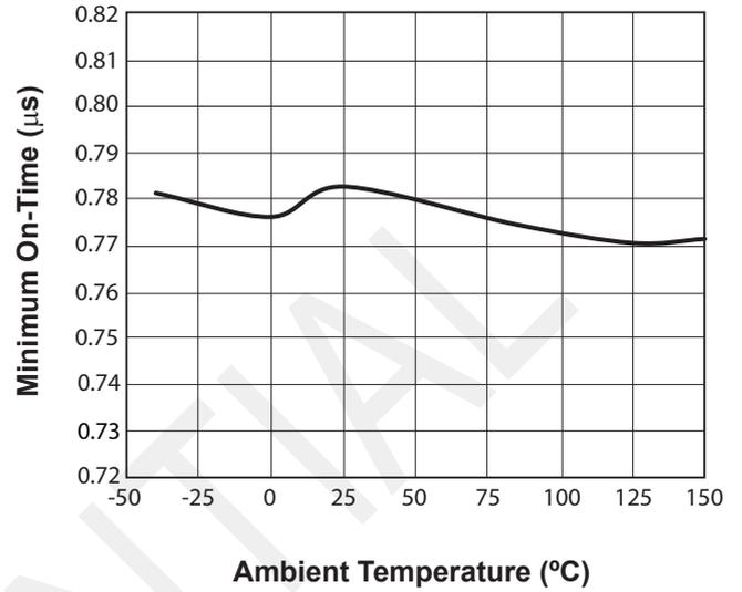
Figure 7.2 : Minimum On-Time vs. Ambient Temperature
