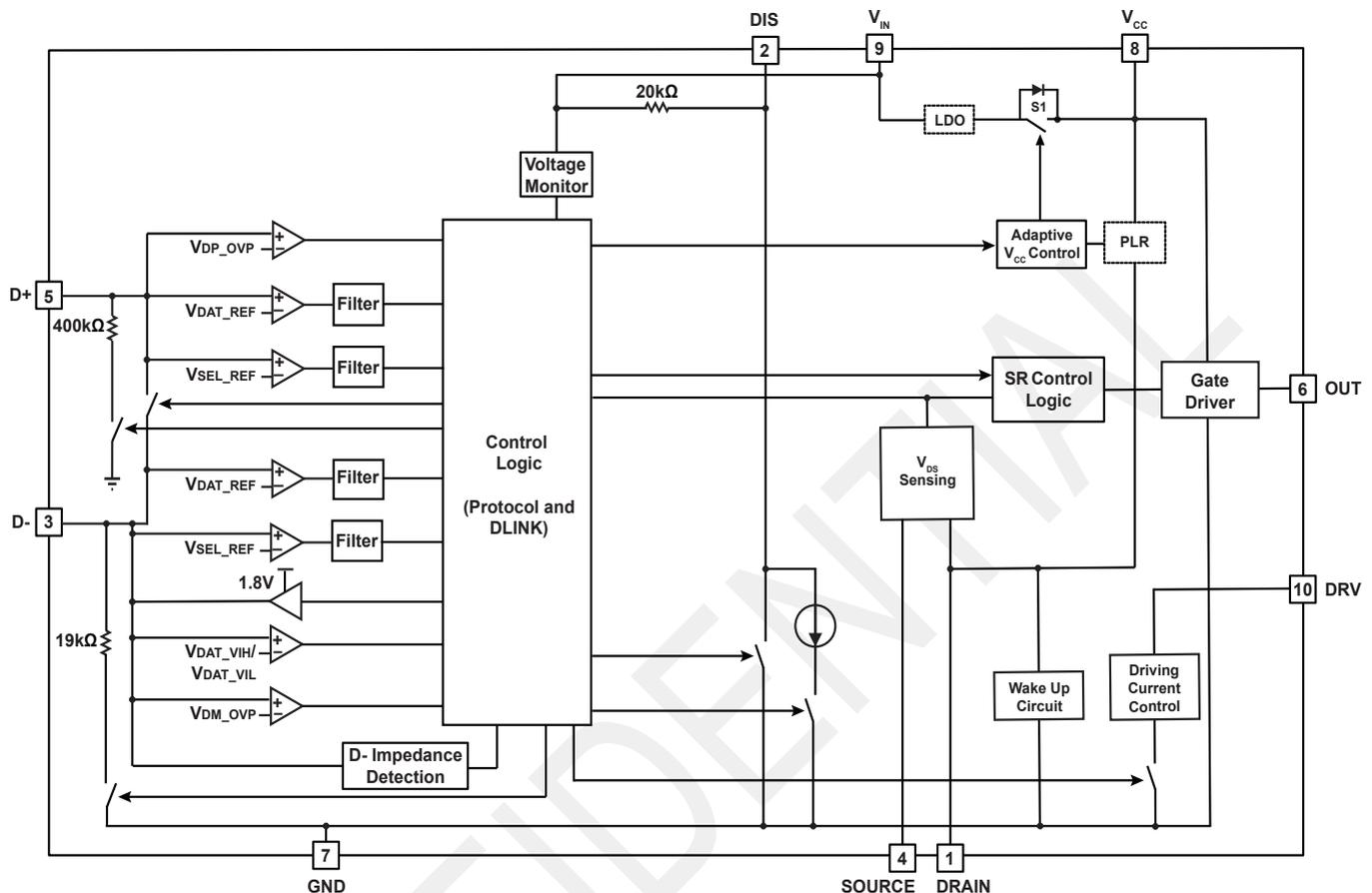
Figure 8.1 : iW661 Functional Block Diagram
