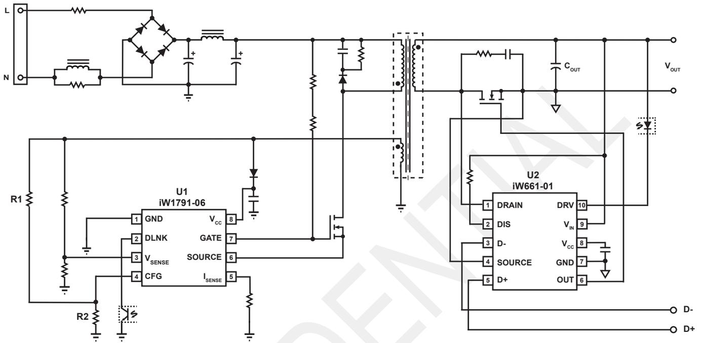
Figure 3.1 : iW661 15W Typical Application Circuit for Multi-Level Output Voltage and Current (Using iW1791 as Primary-Side Controller. Achieving < 20mW No-Load Power Consumption.)
