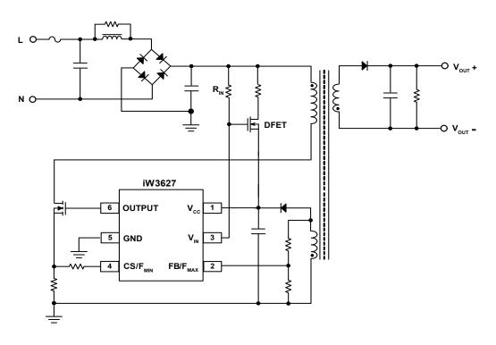
Figure 3.1: iW3627 Typical Application Circuit (Isolated Flyback Application)
