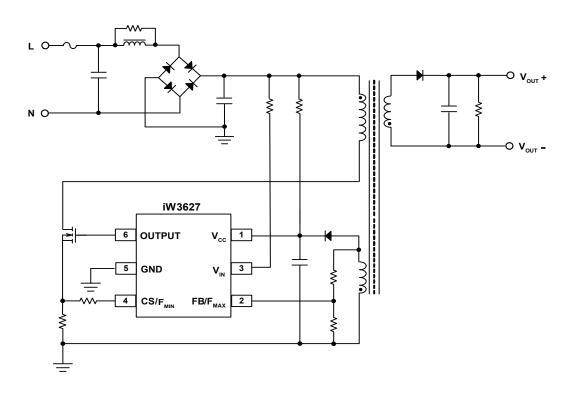
Figure 3.3: iW3627 Typical Application Circuit (Isolated Flyback Application Without Using Active Start-up Device)
