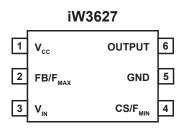
Figure 4.1: 6-Lead SOT23 Package
