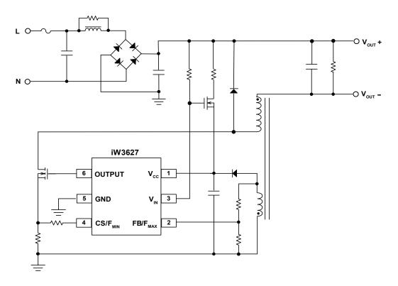
Figure 3.2: iW3627 Typical Application Circuit (Buck Application)
