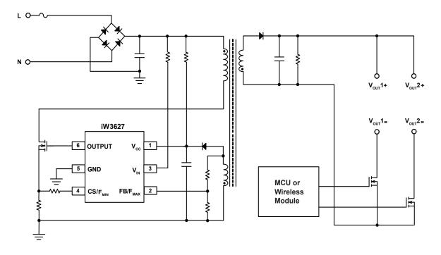
Figure 3.4: iW3627 Typical Application Circuit (Smart Lighting)
