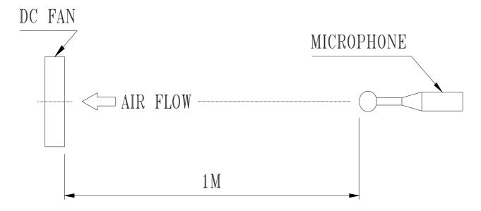
NOISE IS MEASURED AT RATED VOLTAGE IN FREE AIR IN ANECHOIC CHAMBER WITH B & K SOUND LEVEL METER WITH MICROPHONE AT A DISTANCE OF ONE METER FROM THE FAN INTAKE.
