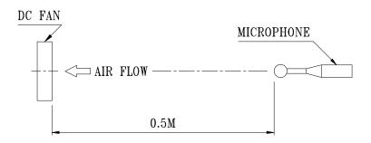
NOISE IS MEASURED AT RATED VOLTAGE IN FREE AIR IN SEMI-ANECHOIC CHAMBER WITH B & K SOUND LEVEL METER WITH MICROPHONE AT A DISTANCE OF 0.5M FROM THE FAN INTAKE. THE NOISE AT 1M SHOULD CALCULATED FROM THE VALUE MEASURED AT 0.5M.
