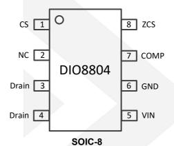
Figure 2 Pin Assignment (Top View)
