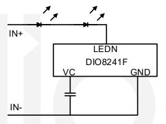
1. The value of the capacitor between VC and GND can determine the final amplitude of the current ripple. It should be large enough in order to remove the current ripple of the LED string. However, too large capacitor may low down the dynamic response.
