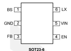
Figure 1 Pin Assignment (Top View)
