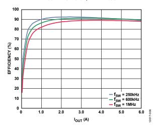
Figure 6. Channel 1/Channel 2 Efficiency Curve,  $V_{\text{IN}} = 12 \text{ V}$ ,  $V_{\text{OUT}} = 3.3 \text{ V}$ , MOSFET = SI4204DY, FPWM Mode
