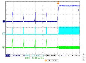
Figure 27. Short-Circuit Protection Recovery,  $V_{IN} = 12 \text{ V}$ ,  $V_{OUT} = 1.2 \text{ V}$ ,  $f_{SW} = 600 \text{ kHz}$ ,  $L = 1 \mu\text{H}$ ,  $C_{OUT} = 47 \mu\text{F} \times 2$ , Channel  $1 = V_{OUTx}$ , Channel 2 = SWx, Channel  $4 = I_{LX}$
