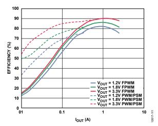
Figure 11. Channel 3/Channel 4 Efficiency Curve,  $V_{IN} = 12 V$ ,  $f_{SW} = 600 \text{ kHz}$ , FPWM and Automatic PWM/PSM Modes
