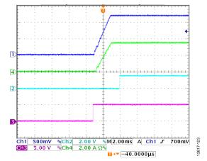
Figure 23. Channel 1 Soft Start with 4 A Resistance Load,  $V_{IN} = 12 \text{ V}$ ,  $V_{OUT} = 1.2 \text{ V}$ ,  $f_{SW} = 600 \text{ kHz}$ ,  $L = 1 \mu\text{H}$ ,  $C_{OUT} = 47 \mu\text{F} \times 2$ , Channel  $1 = V_{OUTI}$ , Channel 2 = PWRGD, Channel 3 = EN1, Channel  $4 = I_{OUTI}$
