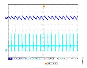
Figure 20. Steady State Waveform at Light Load,  $V_{\text{IN}} = 12 \text{ V}$ ,  $V_{\text{OUT}} = 3.3 \text{ V}$ ,  $I_{\text{OUT}} = 30 \text{ mA}$ ,  $f_{\text{SW}} = 600 \text{ kHz}$ ,  $L = 4.7 \,\mu\text{H}$ ,  $C_{\text{OUT}} = 47 \,\mu\text{F} \times 2$ , Automatic PWM/PSM Mode, Channel  $1 = V_{\text{OUTV}}$ , Channel 2 = SWx
