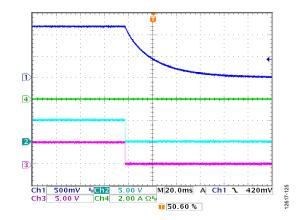
Figure 25. Channel 1 Shutdown with Active Output Discharge,  $V_{IN}=12\,V$ ,  $V_{OUT}=1.2\,V$ ,  $f_{SW}=600\,$  kHz,  $L=1\,\mu$ H,  $C_{OUT}=47\,\mu$ F  $\times$  2, Channel 1 =  $V_{OUT}$ , Channel 2 = EN1, Channel 3 = PWRGD, Channel 4 =  $I_{OUT}$
