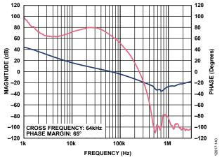
Figure 40. Bode Plot for 1.2 V Output
