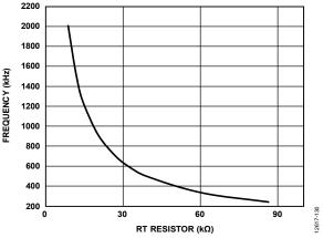
Figure 30. Switching Frequency vs. RT Resistor
