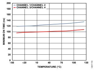
Figure 18. Minimum On Time vs. Temperature
