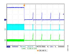
Figure 26. Short-Circuit Protection Entry,  $V_{\text{IN}} = 12 \text{ V}$ ,  $V_{\text{OUT}} = 1.2 \text{ V}$ ,  $f_{\text{SW}} = 600 \text{ kHz}$ ,  $L = 1 \mu\text{H}$ ,  $C_{\text{OUT}} = 47 \mu\text{F} \times 2$ , Channel  $1 = V_{\text{OUTX}}$ , Channel 2 = SWx, Channel  $4 = I_{\text{LX}}$
