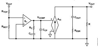
Figure 39. Simplified, Peak Current-Mode Control, Small Signal Circuit
