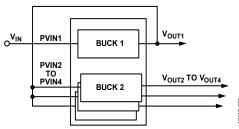
Figure 28. Cascading Supply Application
