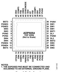
Figure 3. Pin Configuration
