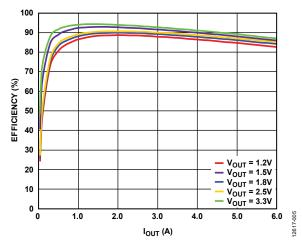
Figure 5. Channel 1/Channel 2 Efficiency Curve,  $V_{IN} = 5 V$ ,  $f_{SW} = 600 \text{ kHz}$ , MOSFET = SI4204DY, FPWM Mode
