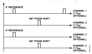
Figure 31. Phase Shift Diagram, Four Buck Regulators
