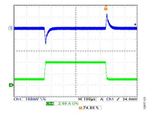
Figure 21. Channel 1/Channel 2 Load Transient, 1 A to 4 A,  $V_{IN}$  = 12 V,  $V_{OUT}$  = 3.3 V,  $f_{SW}$  = 600 kHz, L = 2.2  $\mu$ H,  $C_{OUT}$  = 47  $\mu$ F  $\times$  2, Channel 1 =  $V_{OUTV}$ , Channel 4 =  $I_{OUTX}$
