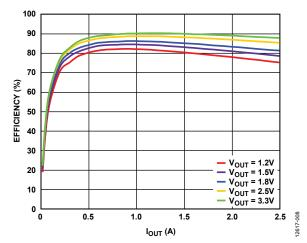
Figure 8. Channel 3/Channel 4 Efficiency Curve, V<sub>IN</sub> = 12 V, f<sub>SW</sub> = 600 kHz, FPWM Mode
