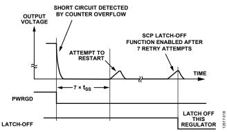
Figure 38. Short-Circuit Latch-Off Detection
