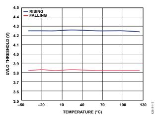
Figure 16. UVLO Threshold vs. Temperature
