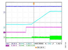
Figure 24. Channel 1 Startup with Precharged Output,  $V_{IN} = 12 V$ ,  $V_{OUT} = 3.3 V$ , Channel  $1 = V_{IN}$ , Channel  $2 = V_{OUT1}$ , Channel 3 = EN1, Channel  $4 = I_{L1}$
