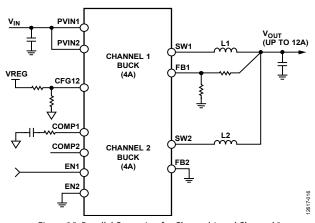
Figure 35. Parallel Operation for Channel 1 and Channel 2 The following considerations apply when two channels are operated in parallel configuration.
