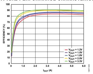
Figure 4. Channel 1/Channel 2 Efficiency Curve,  $V_{IN} = 12$  V,  $f_{SW} = 600$  kHz, MOSFET = SI4204DY, FPWM Mode
