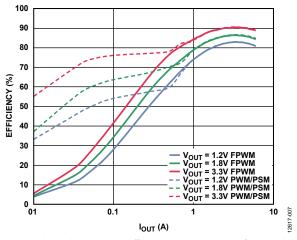
Figure 7. Channel 1/Channel 2 Efficiency Curve, V<sub>IN</sub> = 12 V, f<sub>SW</sub> = 600 kHz, FPWM and Automatic PWM/PSM Modes
