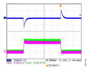
Figure 22. Load Transient, Channel 1/Channel 2 Parallel Output, 0 A to 6 A,  $V_{IN}=12$  V,  $V_{OUT}=3.3$  V,  $f_{SW}=600$  kHz, L=4.7  $\mu$ H,  $C_{OUT}=47$   $\mu$ F  $\times$  4, Channel  $1=V_{OUT}$ , Channel  $3=I_{L1}$ , Channel  $4=I_{L2}$
