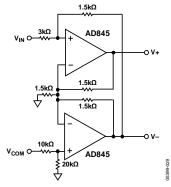
Figure 42. Single-Ended-to-Differential Configuration with the AD845
