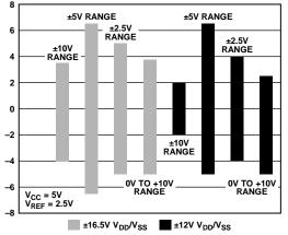
Figure 40. Pseudo Input Range with  $V_{CC} = 5 V$
