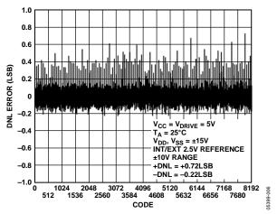
Figure 6. Typical DNL True Differential Mode
