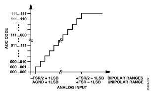
Figure 28. Straight Binary Transfer Characteristic
