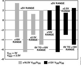
Figure 41. Pseudo Input Range with  $V_{CC} = 3 V$
