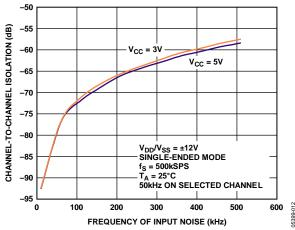
Figure 14. Channel-to-Channel Isolation
