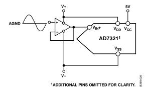
Figure 33. Single-Ended Mode Typical Connection Diagram
