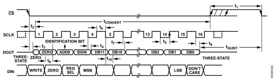
Figure 2. Serial Interface Timing Diagram
