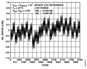
Figure 7. Typical INL True Differential Mode
