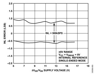
Figure 19. INL Error vs. Supply Voltage at 500 kSPS
