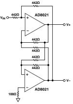
Figure 43. Single-Ended-to-Differential Configuration with the AD8021
