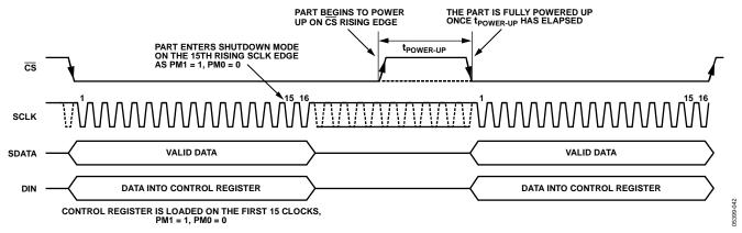
Figure 47. Entering Autoshutdown/Autostandby Mode
