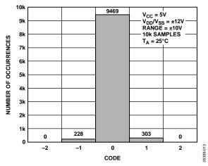
Figure 15. Histogram of Codes, True Differential Mode
