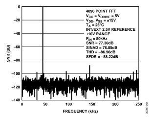
Figure 4. FFT True Differential Mode
