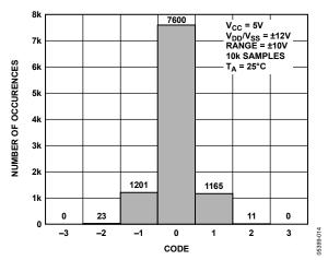
Figure 16. Histogram of Codes, Single-Ended Mode
