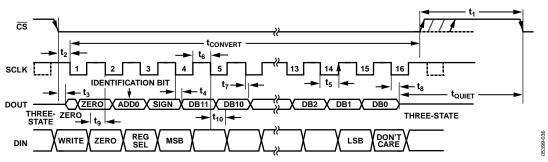
Figure 50. Serial Interface Timing Diagram (Control Register Write)
