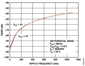
Figure 17. CMRR vs. Common-Mode Ripple Frequency
