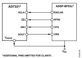
Figure 52. Interfacing the AD7321 to the ADSP-BF53x
