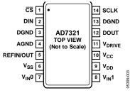
Figure 3. Pin Configuration
