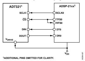
Figure 51. Interfacing the AD7321 to the ADSP-21xx
