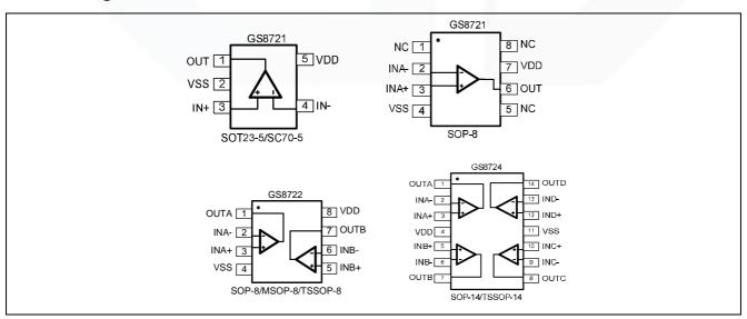
Figure 1. Pin Assignment Diagram
