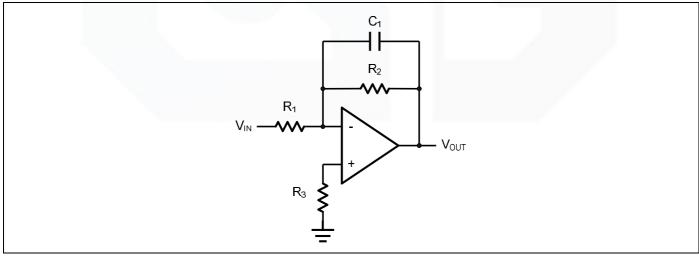
Figure 5. Low Pass Active Filter
