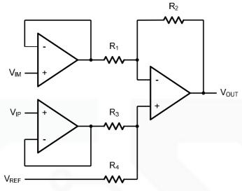
Figure 6. Instrument Amplifier
