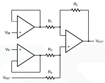
Figure 6. Instrument Amplifier
