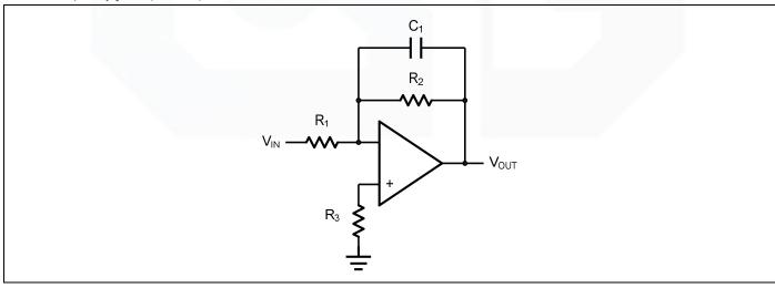
Figure 5. Low Pass Active Filter
