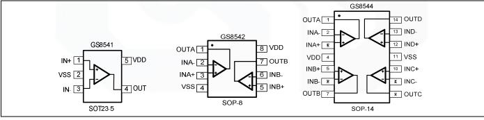
Figure 1. Pin Assignment Diagram
