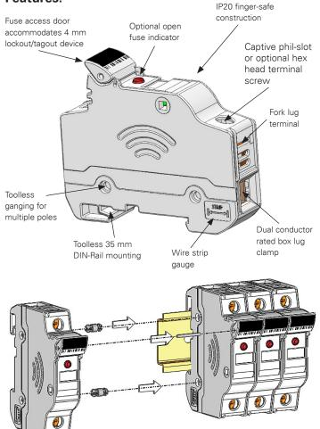
Gang multiple poles to meet application requirements using kit catalog number JV-L (gangs up to four poles).
