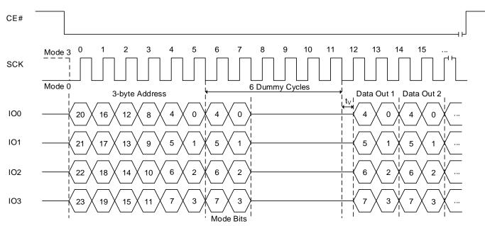
Figure 8.7.2 Fast Read Quad I/O AX Sequence (without command decode cycles)
