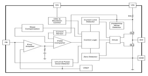
Figure 1. H9008 Block Diagram
