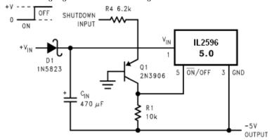
Figure 9. Inverting Regulator Ground Referenced Shutdown
