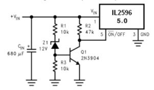
Figure 4. Undervoltage Lockout for Buck Regulator
