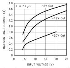
Figure 8. Inverting Regulator Typical Load Current
