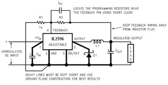
$$V_{OUT} = V_{REF} \left( 1 + \frac{R_2}{R_1} \right)$$
