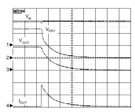
$$\begin{split} &V_{\text{IN}}\!=\!19V,\,R_{\text{LOAD}}\!=\!1\Omega,\,R_{\text{OCSET}}\!=\!1.5k\Omega,\\ &C_{\text{IN}}\!=\!0.1\mu\text{F/X7R},\,C_{\text{OUT}}\!=\!470\mu\text{F/Electrolytic},\\ &C\text{H1:}\,\,V_{\text{IN}},\,10V/\text{Div},\,\text{DC} \end{split}$$
