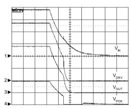
$\begin{aligned} &V_{\text{IN}}\!=\!19\text{V}, \ &R_{\text{LOAD}}\!=\!100\Omega, \ &R3\!=\!51\text{k}\Omega, \\ &C_{\text{IN}}\!=\!0.1\mu\text{F/X7R}, \ &C_{\text{OUT}}\!=\!1500\mu\text{F/Electrolytic}, \\ &C\text{H1: } &V_{\text{IN}}\!, 5\text{V/Div}, \ DC \end{aligned}$
