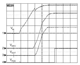
$\begin{aligned} &V_{\text{IN}}\!=\!19V, \ R_{\text{LOAD}}\!=\!100\Omega, \ R3\!=\!\!51k\Omega, \\ &C_{\text{IN}}\!=\!0.1\mu\text{F/X7R}, \ C_{\text{OUT}}\!=\!1500\mu\text{F/Electrolytic}, \\ &CH1: \ V_{\text{IN}}, \ 5V/\text{Div}, \ DC \end{aligned}$
