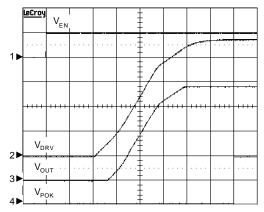
$$\begin{split} &V_{\text{IN}}\!=\!19V,\,R_{\text{LOAD}}\!=\!100\Omega,\,R3\!=\!\!51k\Omega,\\ &C_{\text{IN}}\!=\!0.1\mu\text{F}/\text{X7R},\,C_{\text{OUT}}\!=\!1500\mu\text{F}/\text{Electrolytic},\\ &C\text{H1:}\,\,V_{\text{EN}},\,5V/\text{Div},\,DC \end{split}$$
