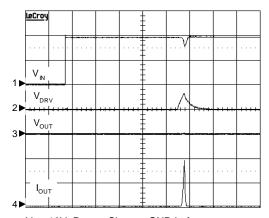
$V_{IN}$ =19V,  $R_{LOAD}$ =Short to GND before power-up,  $C_{\text{IN}}^{\text{IN}}$  =0.1 $\mu$ F/X7R,  $C_{\text{OUT}}$  =470 $\mu$ F/Electrolytic CH1:  $V_{\text{IN}}$ , 10V/Div, DC
