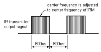
Fig.-1 Transmitter Wave Form
