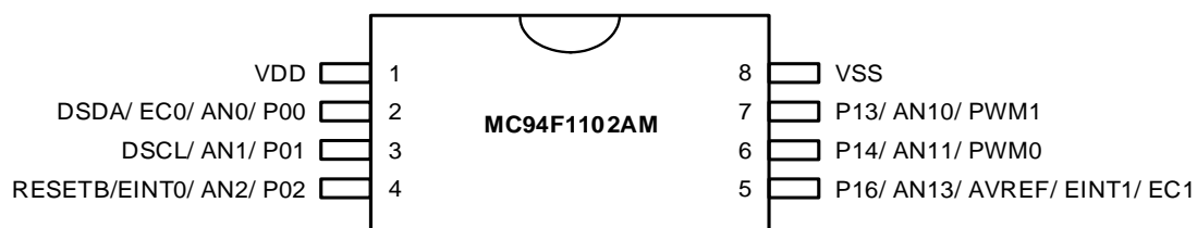
Figure 3.3 MC94F1102AM8 pin assignment
