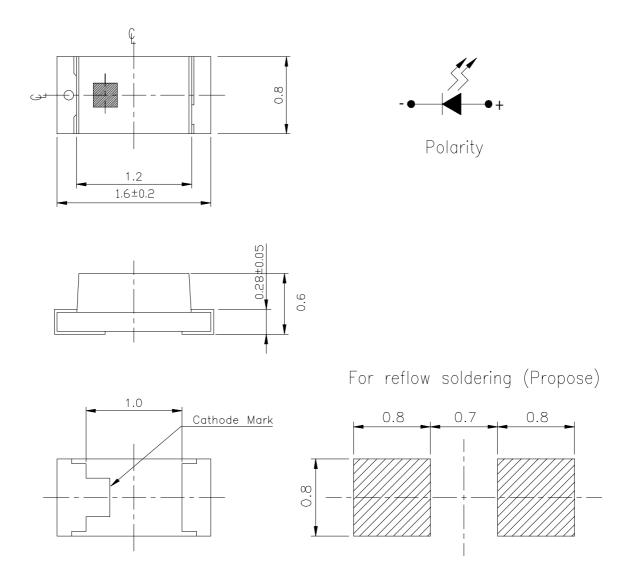
**Note:** Tolerances Unless Dimension is  $\pm 0.1$  mm ,Unit = mm
