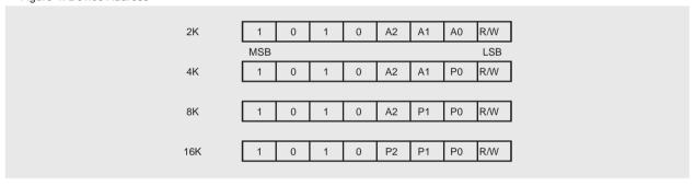
Figure 5: Byte Write
