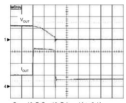
$\boldsymbol{C}_{\text{OUT}} {=} 10 \mu\text{F}, \, \boldsymbol{C}_{\text{IN}} {=} 10 \mu\text{F}, \, \boldsymbol{I}_{\text{OUT}} {=} 1\text{A to } 3.4\text{A}$
