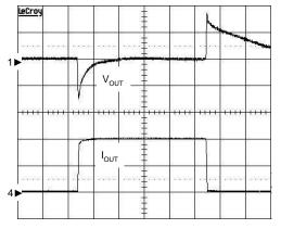
$I_{\text{OUT}}\!\!=\!\!10\text{mA}$  to 2A to 10mA (rise / fall time = 1µs)
