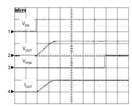
$\begin{array}{l} C_{\text{OUT}} \! = \! 10 \mu \text{F}, \, C_{\text{IN}} \! = \! 10 \mu \text{F}, \, R_{\text{L}} \! = \! 0.6 \Omega \\ \text{CH1: V}_{\text{EN'}}, \, 5 \text{V/Div, DC} \\ \text{CH2: V}_{\text{OUT'}}, \, 1 \text{V/Div, DC} \\ \text{CH3: V}_{\text{POK'}}, \, 5 \text{V/Div, DC} \\ \text{CH4: I}_{\text{OUT'}}, \, 2 \text{A/Div, DC} \\ \text{TIME: 0.5ms/Div} \end{array}$
