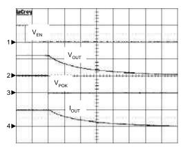
$\begin{array}{l} C_{OUT} \! = \! 10 \mu F, \, C_{IN} \! = \! 10 \mu F, \, R_L \! = \! 0.6 \Omega \\ CH1: \, V_{EN}, \, 5 V/Div, \, DC \\ CH2: \, V_{OUT}, \, 1 V/Div, \, DC \\ CH3: \, V_{POK}, \, 5 V/Div, \, DC \\ CH4: \, I_{OUT}, \, 2 A/Div, \, DC \\ TIME: \, 5 \mu s/Div \end{array}$
