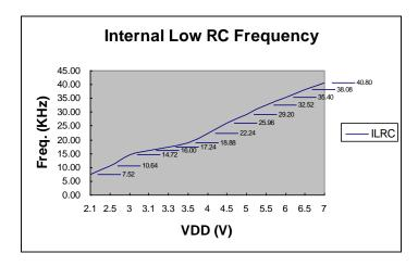
The internal low RC supports watchdog clock source and system slow mode controlled by "CLKMD" bit of OSCM register.
