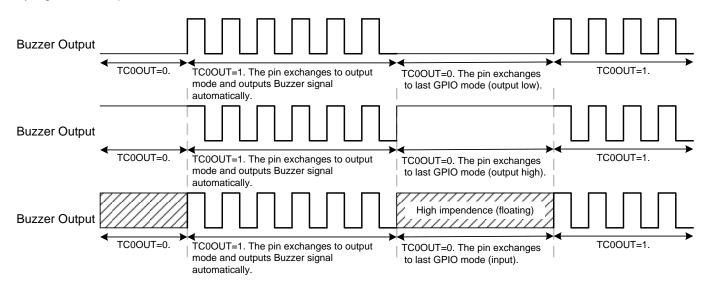
Note: Because the TC0OUT decides the PWM cycle in PWM mode. The PWM0OUT bit must be "0" when buzzer output function works.
