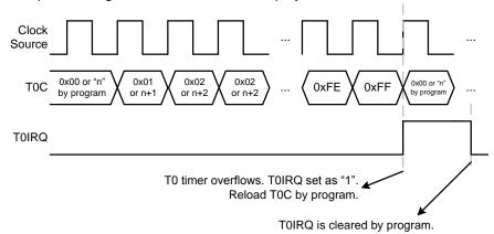
T0 clock source is Fcpu (instruction cycle) through T0rate[2:0] pre-scaler to decide Fcpu/2~Fcpu/256. T0 length is 8-bit (256 steps), and the one count period is each cycle of input clock.
