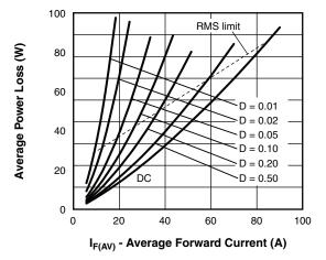
Fig. 6 - Forward Power Loss Characteristics
