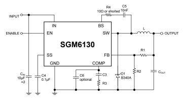
Figure 2. Typical Application Circuit
