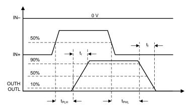
图 18. OUTH and OUTL Propagation Delay, Noninverting Configuration
