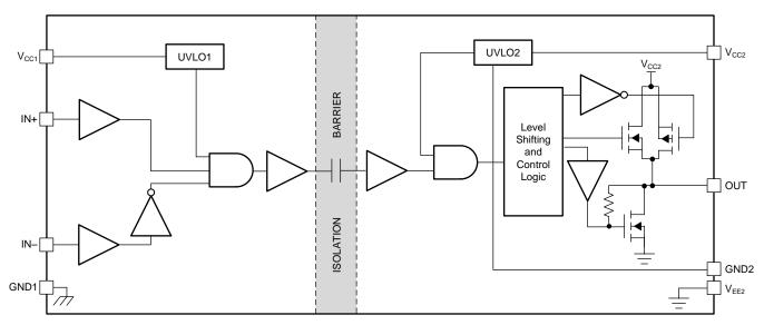
图 27. Functional Block Diagram—UCC5320E and UCC5390E UVLO With Respect to GND2
