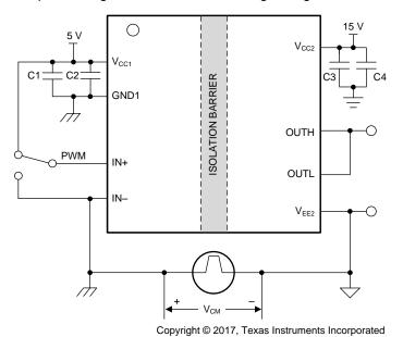
图 20. CMTI Test Circuit for UCC5320S and UCC5390S
