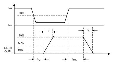
图 19. OUTH and OUTL Propagation Delay, Inverting Configuration
