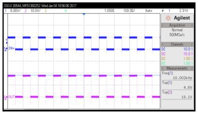
$V_{CC2} = 20 \text{ V}$   $V_{EE2} = \text{GND}$   $f_{SW} = 10 \text{ kHz}$  图 40. PWM Input And Gate Voltage Waveform
