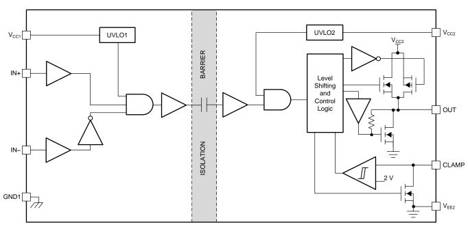
图 26. Functional Block Diagram—UCC5310M and UCC5350 Miller Clamp
