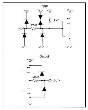
图 33. Device Input and Output Structure
