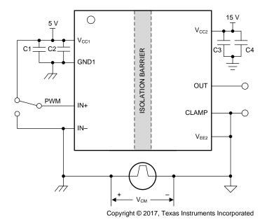
图 21. CMTI Test Circuit for UCC5310M and UCC5350M
