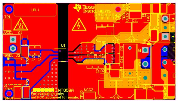
(1) No PCB traces or copper are located between the primary and secondary side, which ensures isolation performance.
