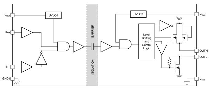
图 25. Functional Block Diagram—UCC5320S and UCC5390S Split Outputs
