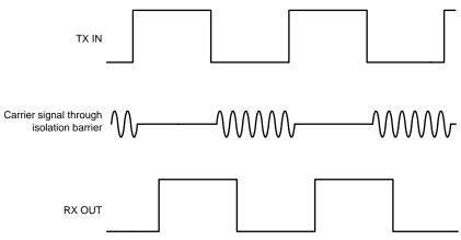
图 24. On-Off Keying (OOK) Based Modulation Scheme
