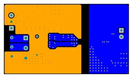
图 43. Bottom-Layer Traces and Copper (Flipped)
