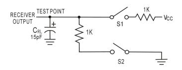
Figure 2. Receiver Enable/Disable Timing Test Load
