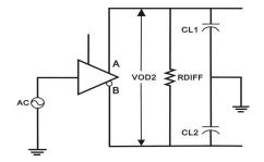
Figure 3. Driver Timing Test Load
