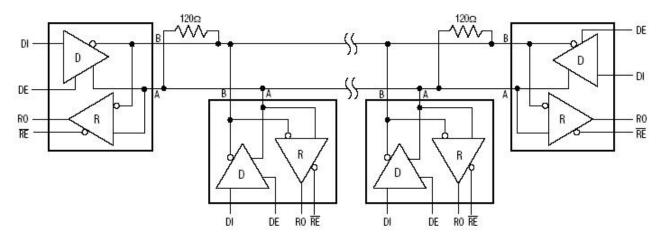
Figure 10. GM3085E Pin Configuration and Typical Half-Duplex Operating Circuit
