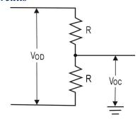
Figure 1. Driver DC Test Load
