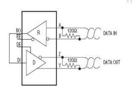
Figure 8. Line Repeater for GM3085E
