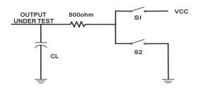
Figure 4. Driver Enable/Disable Timing Test Load
