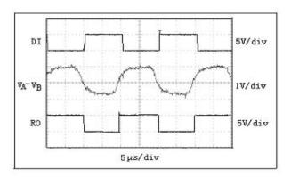
Figure 9.GM3085E System Differentia Voltage at 50 kHzDriving 4000ft of Cable
