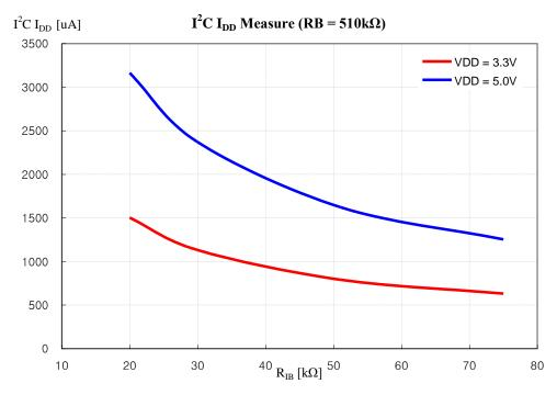
I2C Block operation current consumption curve
