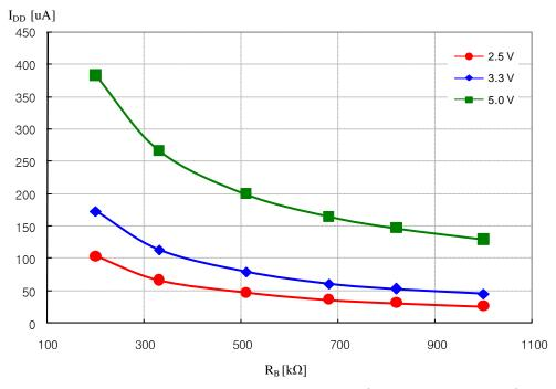
Normal operation current consumption curve (Pin21 I2C\_EN is High)
