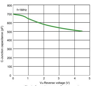
Fig 4. Capacitance vs. Reveres voltage
