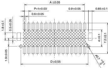
Note 1:Shaded area must be free of any electrically conductive traces to avoid contact with soldered pin header terminations. Note 2: Required only for pin headers supplied with the positioning boss.
